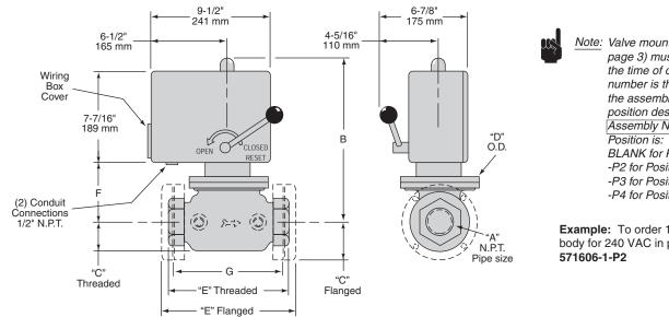
Note: Valve mounting position (see page 3) must be specified at the time of order. The part number is the combination of the assembly number and the position designator. Assembly No. Position BLANK for Position #1 -P2 for Position #2 -P3 for Position #3 -P4 for Position #4
